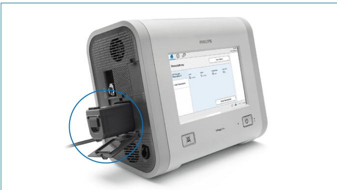
7. Reconnect the detachable battery and AC power source.
